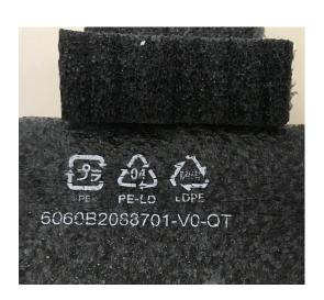
Samples of extruded sheet which have been cut and joined to make shapes to protect products.
