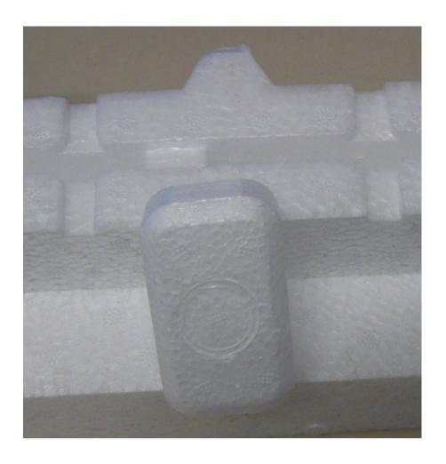
Sample of expanded polypropylene, showing the polymer identification code and fractured surface
