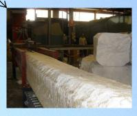
The EPS is compacted to increase the density by up to 20 times using a screw compactor.
