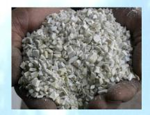
Wash & Granulate After an initial wash the plastic is further reduced in size to granules less than 15 mm. It is then rewashed and dried.
